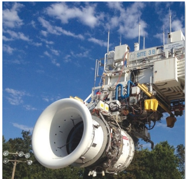
CFM INTERNATIONAL , a joint venture between Snecma (Safran) and GE, initiated testing of the first full LEAP engine in September. The engine includes 19 3D printed fuel nozzles.
